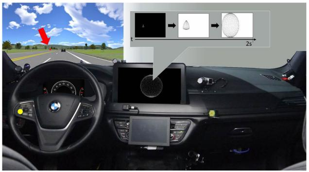
**Fig. 1.** Car-following task in the simulator. The red dot represents the visual DRT in study 2. The animations are displayed in the CID. An example of a 2s animation containing attention capturing properties is shown.
