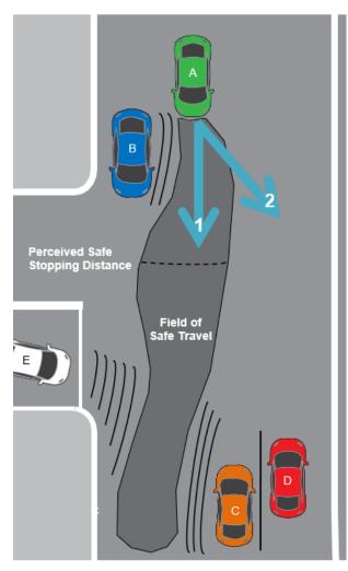
**Fig. 1.** FoST illustration for a driver approaching an intersection. Assumes left-hand drive. Vehicle A represents ego vehicle. Driver attention can be directed straight ahead (scenario 1) or off-road to the right (scenario 2).
