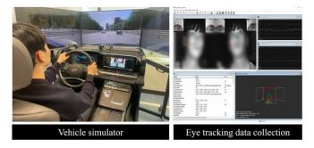
Fig. 2. Vehicle simulator environment
