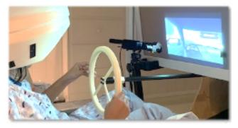
*Fig 1. Exemplar participant using the driving simulation in the MEG laboratory with MEG-compatible eye-tracker.*
