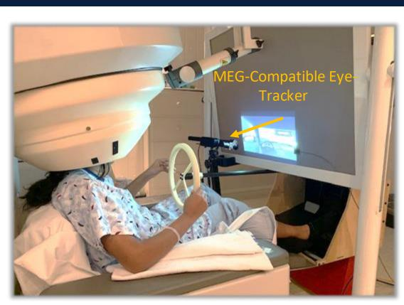
Participants seated in a CTF-Omega 275 Channel MEG (600 Hz) Included MEG-compatible eye-tracker (SR Research EyeLink 1000; 1000) Hz) and driving hardware (Current Designs, Inc.)
