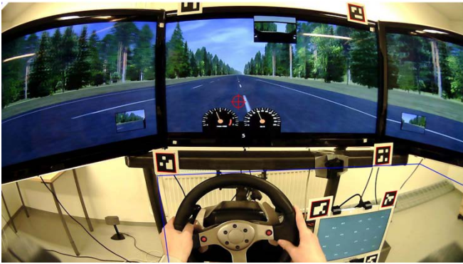
Figure 1: The setup of the experiment illustrating a visually and cognitively high-demanding secondary task (Grahn et al., 2023)
