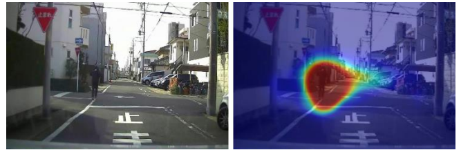
Fig. 1. Left: Dashcam image. Right: Driver's Focus of Attention (DFoA) as predicted when using the driver attention predictor trained with conventional dataset. While it can detect the pedestrian, it should also consider traffic signs, blind spots, etc. in this complex environment.
