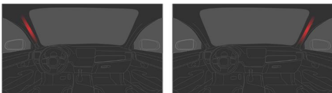
Figure 1: illustration of the location and shape of ambient light that showed the approach or breach of the lane line or lane edge.
