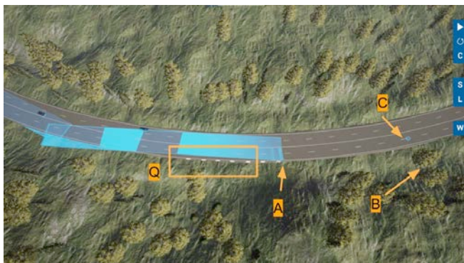
Fig. 1. The traffic area with a maximum of 70 km/h. [Q] warning zoon, [A] warning activation, [B] object
