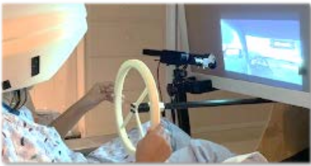
Fig 1. Exemplar participant using the driving simulation in the MEG laboratory with MEG-compatible eye-tracker.
