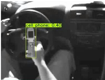
Fig. 2. Detected cell phone use of a driver by YOLOv4
