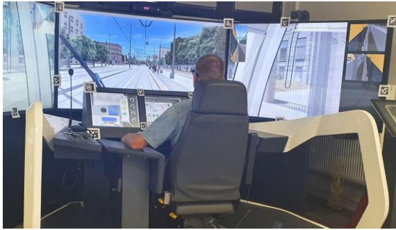
Fig. 1. Study settings. Driver operates the simulator while wearing eye-tracking glasses
